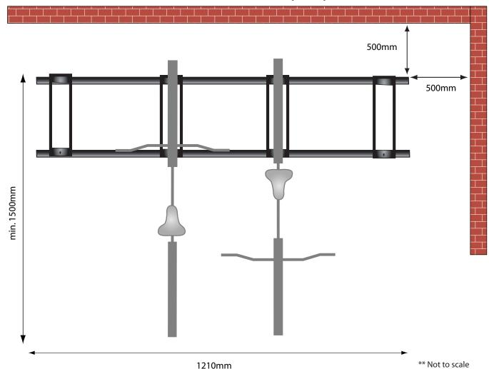
To fix permanently to cement, use 8mm dynabolt in the holes provided.
